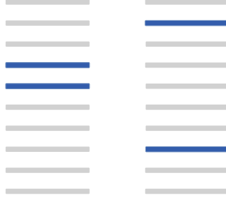
Fig. 1. Two rankings (with two positives and eight negatives examples) ordered from the highest score (at the top) to the lowest. On the left, we get AUCROC = 0.63 and AP = 0.33 . On the right, AUCROC = 0.56 and AP = 0.38 . Therefore, the two criteria disagree on the best ranked list. (Color figure online)
