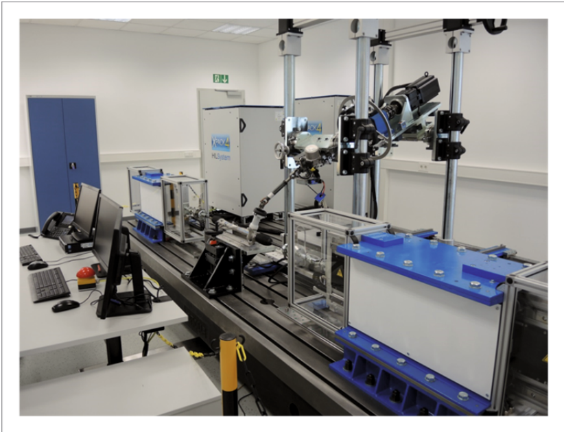
Figure 8: Hardware-in-the-Loop Steering Test Bench at HMETC
