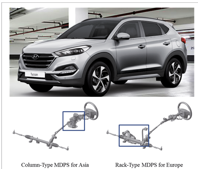
Figure 6: Comparison of Column-MDPS and Rack-MDPS
