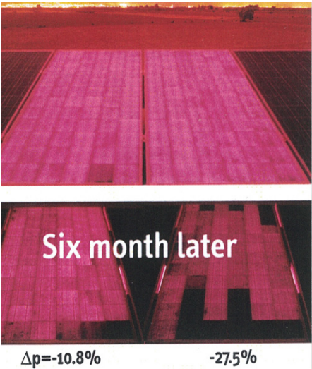
Fig. 4 Degradation of PV modules due to PID resulting in loss of power (Source: PI-Berlin)
