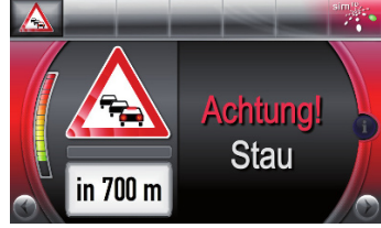
(b) Traffic jam ahead. Based on Decentralized Environmental Notification Messages (DENMs), which may be forwarded over multiple hops.
