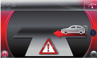
(a) Intersection collision avoidance: Approaching vehicle from the right, detected by its Cooperative Awareness Messages (CAMs).
