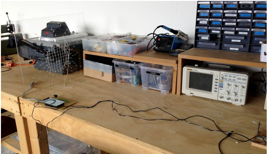
Figure 6: Structure for testing the translation of the electric signal into a mechanical pull (own picture).
