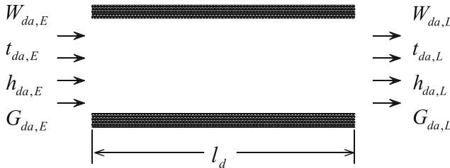
Fig. 2.22 Schematic diagram for straight air duct
