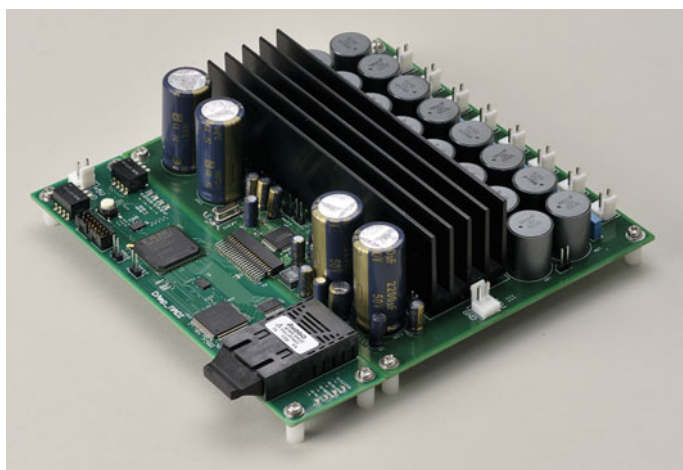
Fig. 2.4 Newly designed 8ch digital amplifiers with a MADI interface
