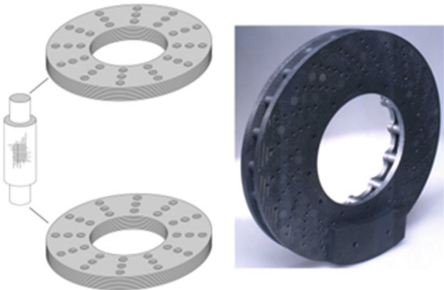
Fig. 13 C/SiC brake disc prototype as an assembly of the single components. The pins connect the frictional surfaces and transfer the heat to the ventilated core of the brake disc [17]
