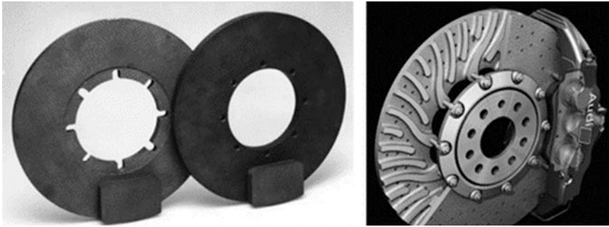
Fig. 11 First generation of 2D-fabric reinforced C/SiC brake discs ( left : DLR) and one current design of ventilated C/SiC brake discs with short fiber reinforcement ( right : Audi AG)
