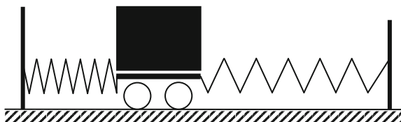
Fig. 2.2 One-dimensional oscillator driven by mechanical springs: the mass-spring system
