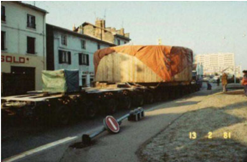
Fig. 2.5 The diaphragm (8.9 m in diameter) passing through a village
