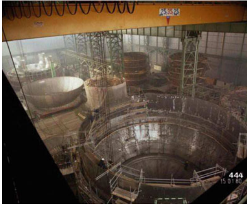
Fig. 2.13 In-workshop manufacturing of the main vessel, of the B1 baffle and, at the back, of inner vessel structures
