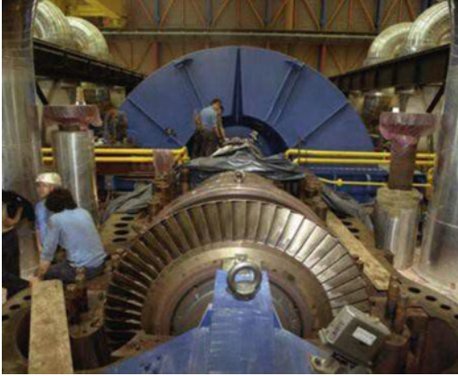
Fig. 2.32 Assembling the last high-pressure stage of one of the two turbines
