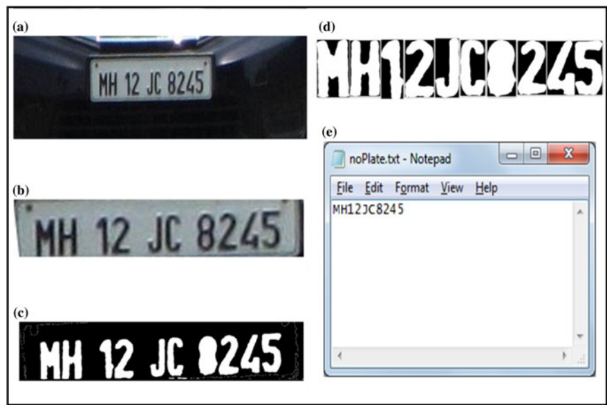
Fig. 4 a Sample image Fig. 2, b Extracted plate, c Processed image, d Extracted letters, e Extracted characters in text file
