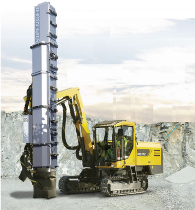
Fig. 2.31 Silenced drilling rig (Reproduced with the permission from Atlas Copco)
