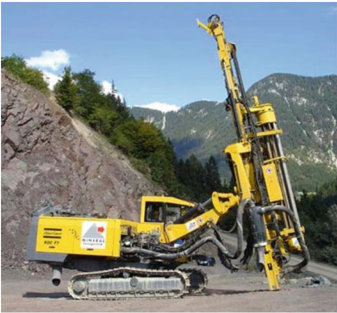
Fig. 2.27 COPROD drill string (Reproduced with the permission from Atlas Copco)
