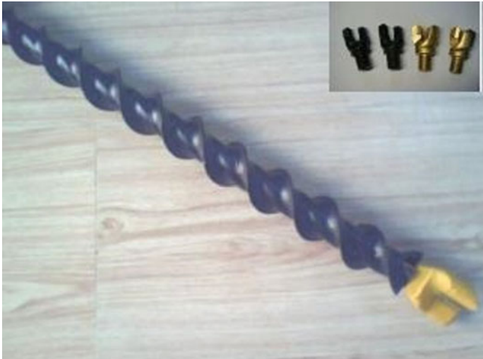
Fig. 2.38 Auger drill with two-wing drag bit
