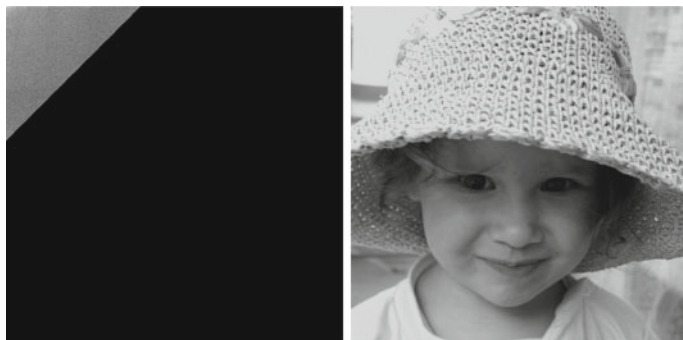
Fig. 2.39 Reconstruction using 8% of the WHT coefficients at 27.09 dB PSNR
