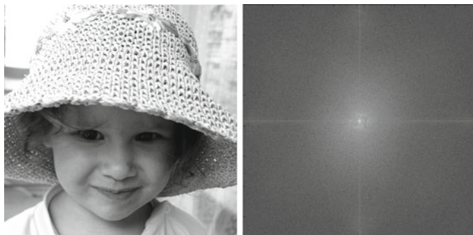
Fig. 2.11 DFT representation of a graylevel image by applying an FFT
