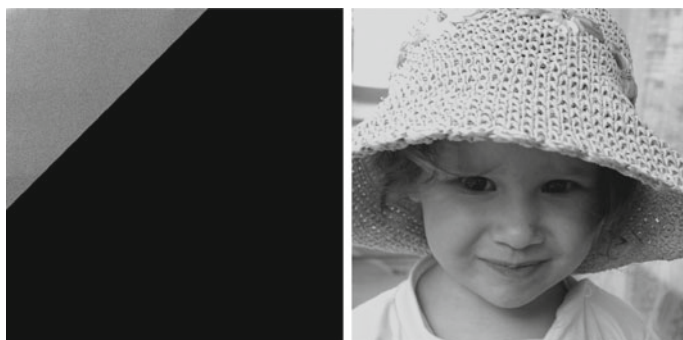
Fig. 2.40 Reconstruction using 18% of the WHT coefficients at 30.27 dB PSNR
