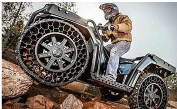
Fig. 2.35 Even elastic tires can better control deformation compatibility and even stress of wheel hubs than the rubber pneumatic tires
