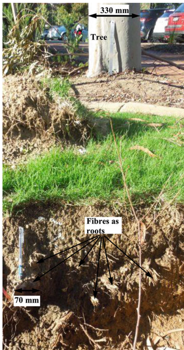
Fig. 2.1 Foundation soil reinforced randomly with natural root fibres (visible in an excavated trench closer to the tree) supporting a tree
