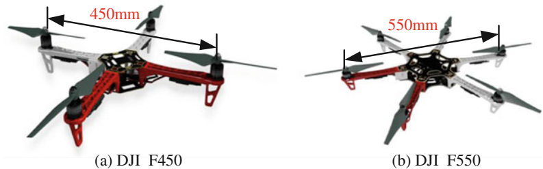
Fig. 2.5 Diagonal size of multicopters
