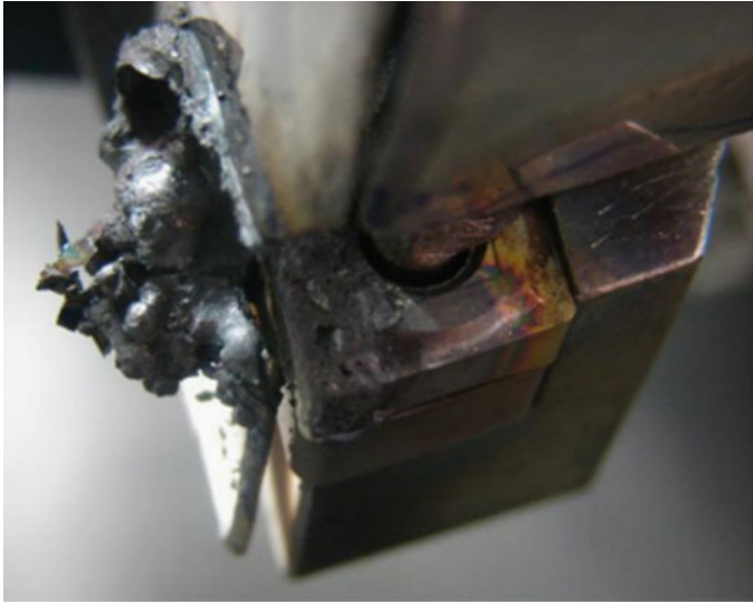
Fig. 7 Damage in the cutting tool when the laser beam is focused at a circumferential distance of 25 mm from the cutting tool [132]
