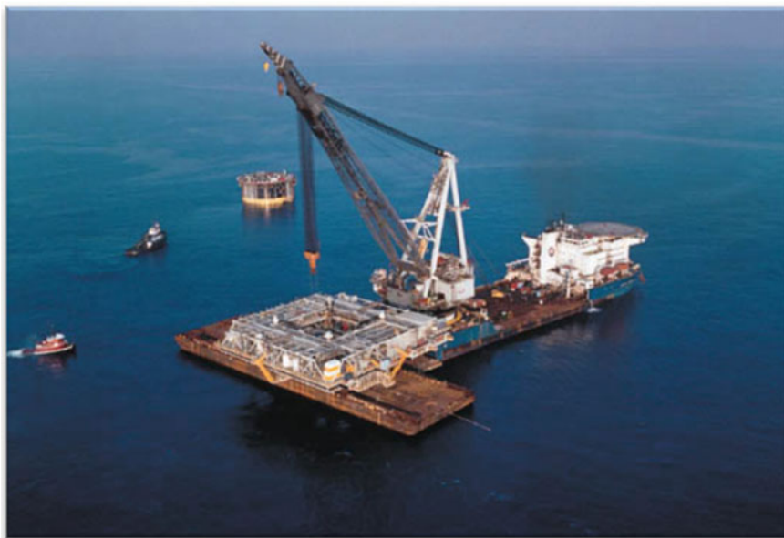
Fig. 2.52 The McDermott DB-50 was preparing to lift up the lower deck of the Genesis spar topsides (courtesy of McDermott)
