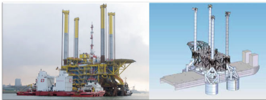
Fig. 2.14 After the leg stiffening frame together with the suction pile is welded to each leg and the platform is ready to sail to the offshore site. It can be seen in the right that the whole 13 m long suction pile is submerged in the water (courtesy of iv-Oil and Gas)
