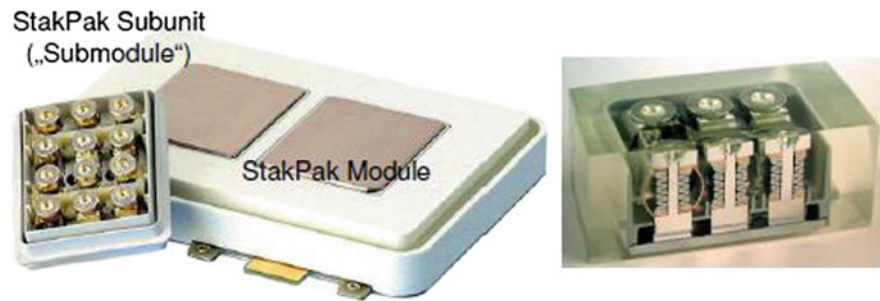
Fig. 2.1 Press-pack IGBT module
