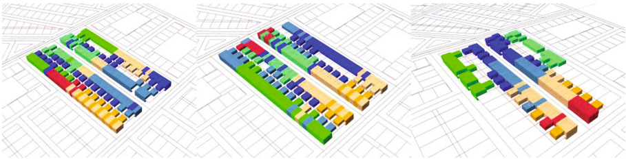
Fig. 13. Clustering of placed buildings. The method allows the designer to allocate residents according to their neighborhood preferences.
