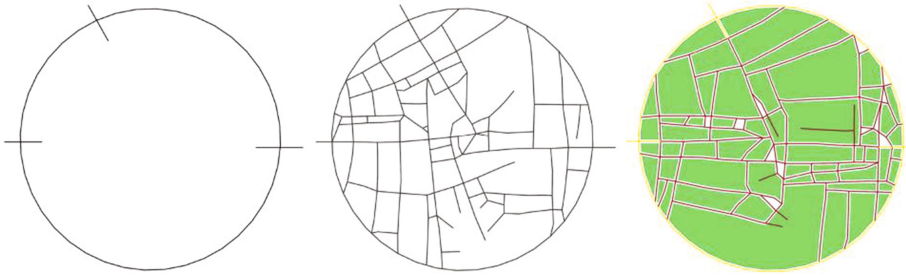
Fig. 6. From a generated street network (component A shown in Fig. 4) with a custom border input B and three custom initial street segments IS , the street blocks are generated on the right side using the component B shown in Fig. 4
