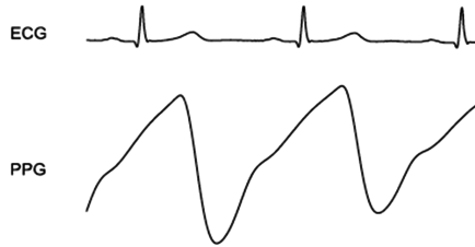
Fig. 1. The pulsatile (AC) component of the PPG signal and corresponding electrocardiogram (ECG). The AC component is actually superimposed on a much larger quasi-DC component that relates to the tissues and to the average blood volume within the sample. It represents the increased light attenuation associated with the increase in microvascular blood volume with each heartbeat.
