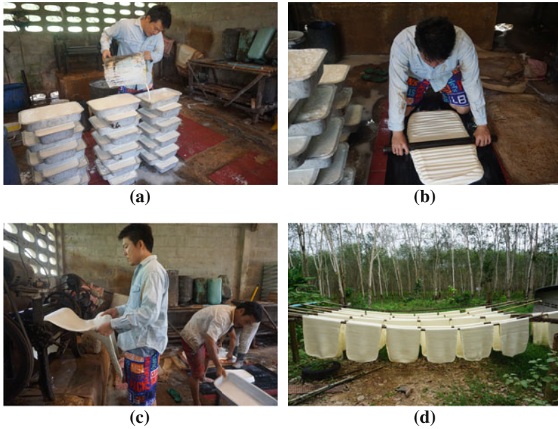
Fig. 2.6 Unsmoked sheet production process
