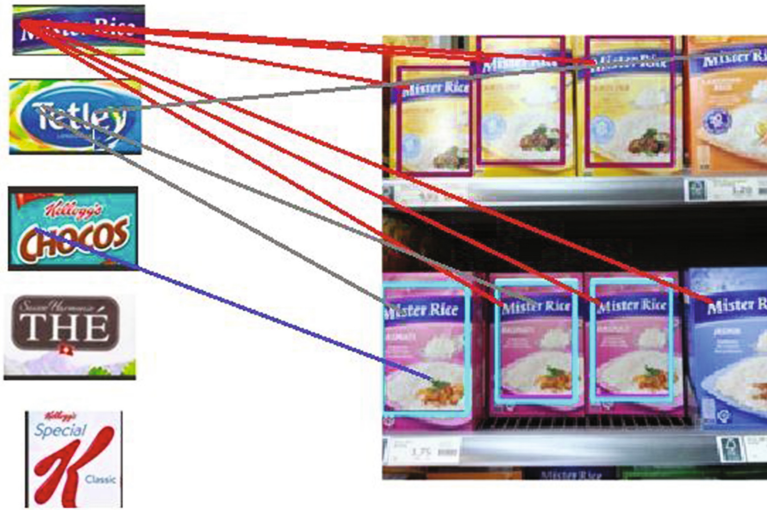
Fig. 2. A pictorial illustration of choosing the top k logos in the logo detection step. The red lines depict the matches between the keypoints in the shelf and the first logo. Similarly, the grey and the blue lines are matches with the next two logos
