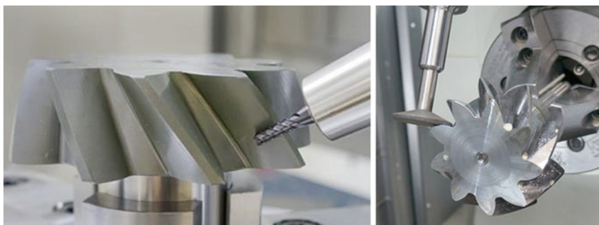
Fig. 10 Rough-cutting and finish-grinding of IPB pinion teeth
