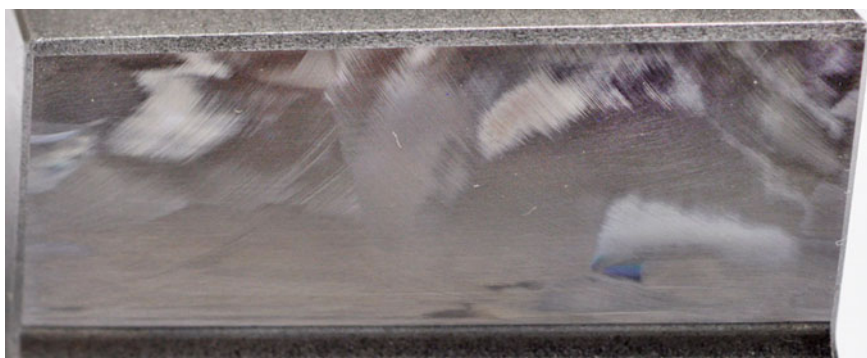
Fig. 19 Plane tooth flank of an IPB wheel finished by one path with a CBN disk tool
