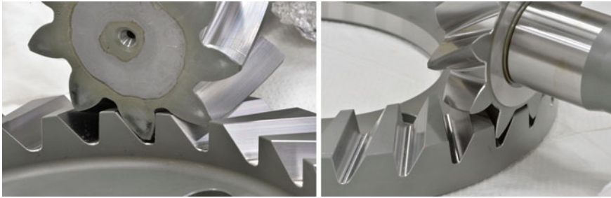
Fig. 24 IPB gears in good mesh and smooth working
