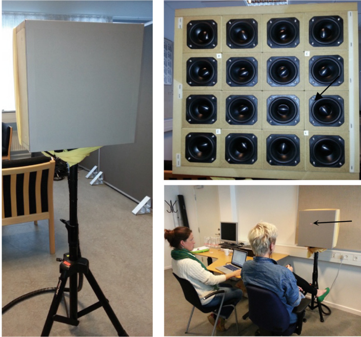
Fig. 1. Left: loudspeaker device used in the experiment. Top right: close-up of the 16 individual speakers without the cover. Bottom right: facilitator with computer and respondent pointing with the laser at the speaker device (laser dot at arrow)
