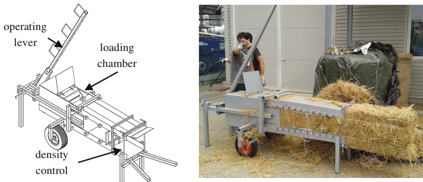
Fig. 9. Press with continuous bale production and slider crank actuation mechanism: detailed design and prototype
