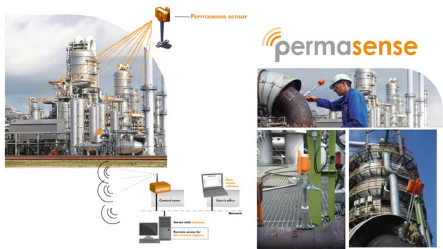
Fig. 1 Overview and pictures of the Permasense Ltd. wireless ultrasonic corrosion monitoring system
