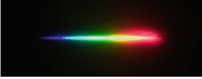
Fig. 2.4 Real image of white light continuum generated in our setup
