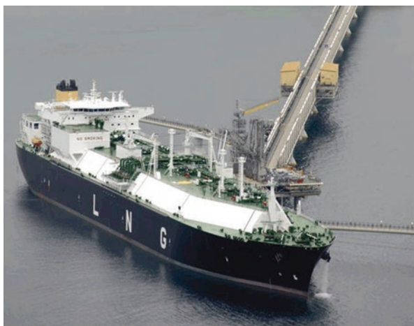
Fig. 2.1 130,000 m 3 LNG carrier with integrated Invar tank
