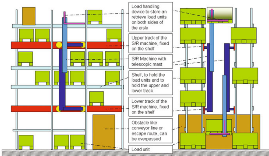
Fig. 1 Sketch of the innovative S/R machine with elevated tracks
