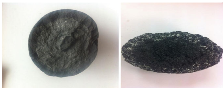
Fig. 2.28 Brex with a layer of fine fraction on the surface. Left: coal (surface layer) and fine fraction of construction materials. Right: coke brex with epoxy resin as binder
