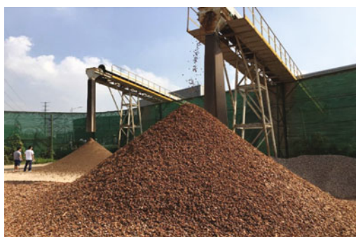
(a) The production line of recycled aggregates
