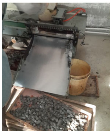
Fig. 2.99 Photographs of manufacture process of sintered abrasive blocks with high temperature. a Extrusion forming materials; b sintered product
