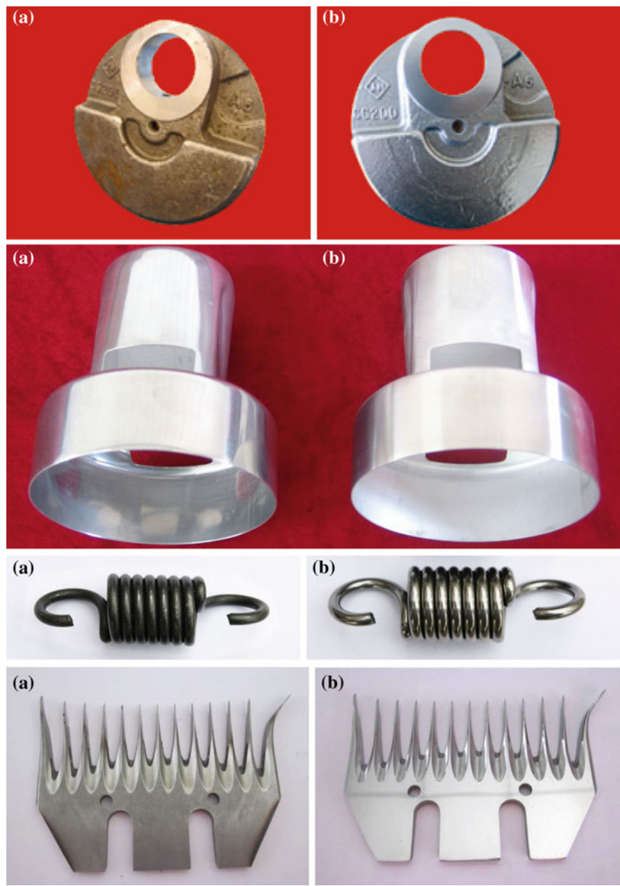
Fig. 2.115 Comparison photographs of miscellaneous parts with small sizes. a Before finishing; b after finishing
