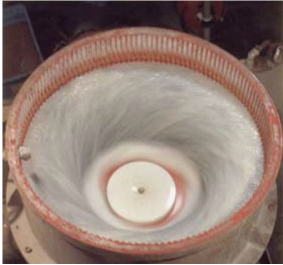
Fig. 2.14 Motion state photograph of whirling barrel finishing process
