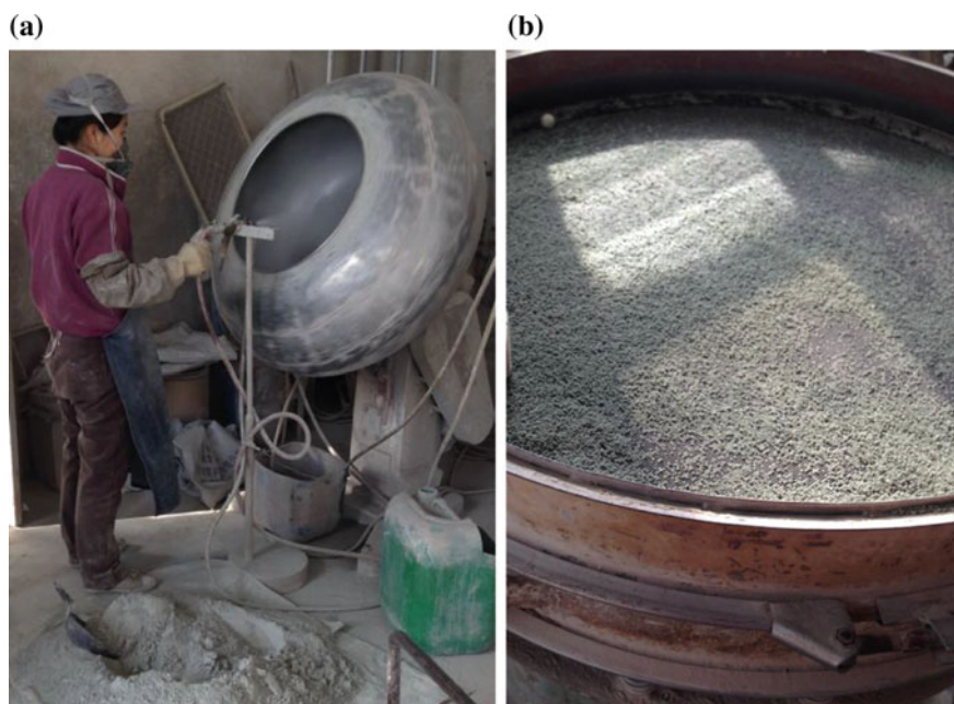
Fig. 2.100 Photographs of manufacture process for spherical abrasive blocks. a Spherical forming; b screening
