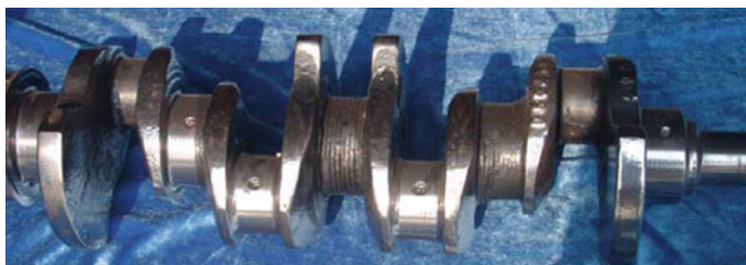
Fig. 2.88 Finishing effect of the crankshaft in long time with one kind of abrasive blocks
