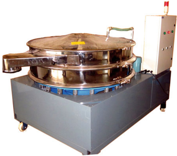
Fig. 2.96 Photograph of abrasive blocks rinsing device
