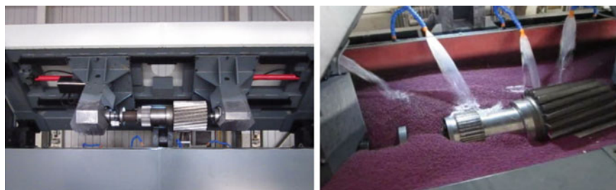
Fig. 2.124 Finishing status of gear shaft with large gear module
