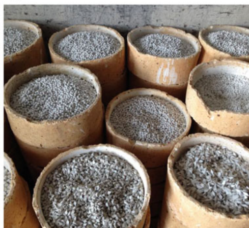
Fig. 2.99 Photographs of manufacture process of sintered abrasive blocks with high temperature. a Extrusion forming materials; b sintered product
