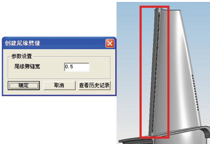
Fig. 2.46 Feature model of trailing edge slot
