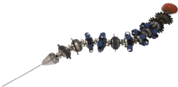
Fig. 2.26 A wheelless pipeline inspection system
