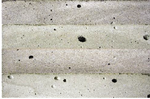
Fig. 8. Voids with various sizes in four SHCC sections sampled from a coupon specimen (Li and Wang 2006).
