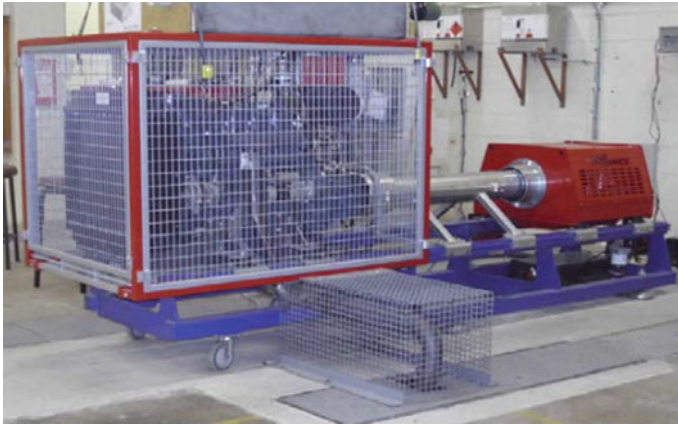
Fig. 3 Engine test bed
