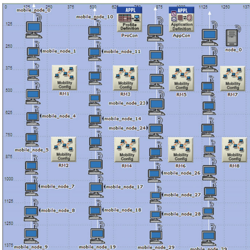
Fig. 2 An example of network model design of MANET using 40 nodes
