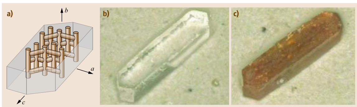
Fig. 19.26a–c An illustration of ZSM-5 zeolite with magnified pore arrangements (a), and photographs of the zeolite (b) and a Se-loaded one (c), the dimension being \approx 40\ \mu\text{m} \times 40\ \mu\text{m} \times 200\ \mu\text{m} . ZSM-5 is a fairly non-polar zeolite with a composition of \text{Si}_{94}\text{Al}_2\text{O}_{192} , containing channels with diameters of \approx 0.7\ \text{nm} (Reprinted from [19.446] with the permission of AIP Publishing)
