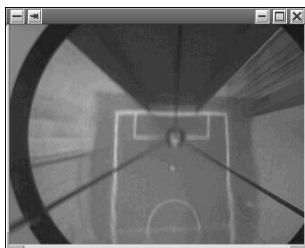
Fig. 5. Omni-directional catadioptric vision image taken by the goalkeeper
