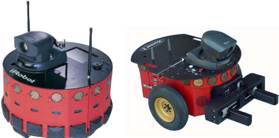
Fig. 7. The Magellan Pro and Pioneer II mobile robots used in the experiments discussed here.
