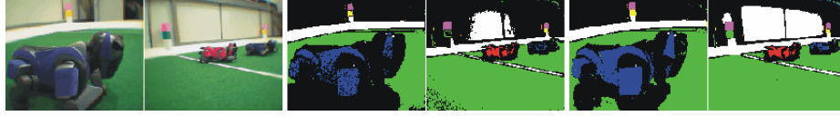
Fig. 4. Color classification of two camera images (left) as done by a conventional YUV-approach (middle) compared with an optimized classification (right)
