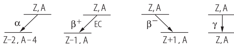
Fig. 3.3. Transmutations of atomic and mass numbers during the main nuclear decay modes.
