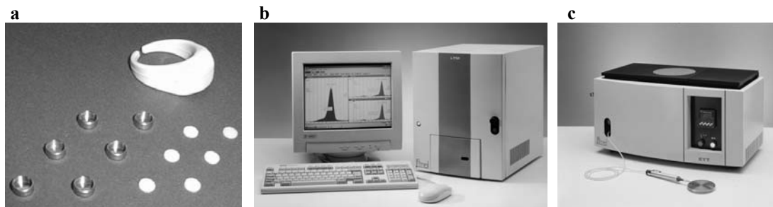
Fig. 10.18. (a) TL detectors for radiation protection measurements (chips, rods, and ring). (b) TLD reader for the evaluation of irradiated detectors. (c) Annealing oven for the preparation of the detectors. TL detectors are placed in a metallic container which comes into contact with two heating plates to ensure optimal thermal equilibrium. (Courtesy PTW Freiburg).
