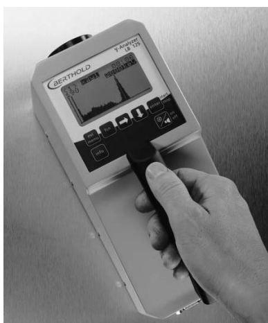
Fig. 10.12. Portable NaI spectrometer with 496 channels for the localization, identification, and measurement of \gamma -rays with an energy between 25 keV and 2 MeV. (Courtesy Berthold Technologies).
