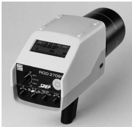
Fig. 10.4 Dose and dose rate survey meter with an air-equivalent ionization chamber (volume 600 \text{ cm}^3 ) for the measurement of X- and \gamma -rays in the energy range between 6 keV and 3 MeV. Using an additional plastic shielding, even photons up to an energy of 7.5 MeV can be measured. The probe is detachable for remote measurements. (Courtesy Step Sensortechnik).
