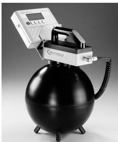
Fig. 10.20. Dose rate monitor (‘rem counter’) for the measurement of neutron ambient dose equivalent H^*(10) for neutrons up to an energy of 20 MeV. The detector system consists of a proportional counter tube centered in a moderator sphere with a diameter of 250 mm. (Courtesy Berthold Technologies).
