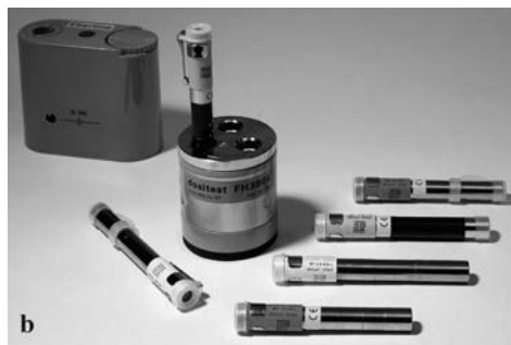
Fig. 10.6. Pen-size direct-reading ion chamber dosimeter for personal radiation protection measurements in a \gamma - or X-ray environment. (a) Simplified schematic representation. (b) Pocket dosimeters for different dose and energy ranges. The nominal voltage required to 'set the dosimeter to zero' is adjusted with the charging unit (potentiometer). A test source is used to check the correct function and calibration of the personal dosimeters. (Courtesy Thermo Eberline ESM).
