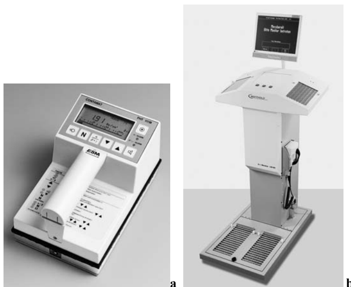
Fig. 10.9. Large-area proportional counters for contamination detection. a: Sealed handheld monitor for detection of surface contaminations with \alpha -, \beta - and \gamma -isotopes. (Courtesy Thermo Eberline ESM). b: Continuous gas-flow contamination monitor for detection of \alpha - and \beta -contaminations of hands, shoes, and clothing. (Courtesy Berthold Technologies).
