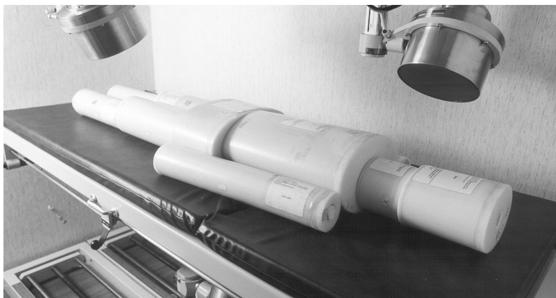
Fig. 10.43. The BOMAB phantom for simulation of homogeneous activity depositions in the whole body
