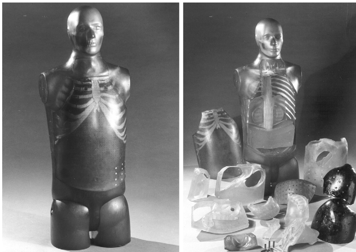
Fig. 10.46. The “Fission product phantom” for simulation of activity depositions in all relevant organs of the trunk (Humanoid Systems Inc.)
