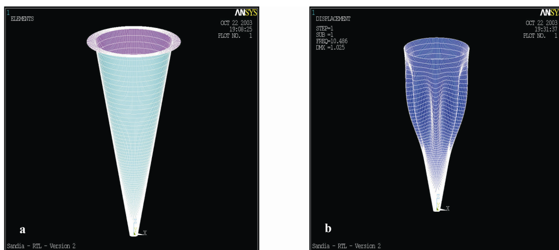
Fig. 9.17. RTL structural properties buckling analysis [03Kam]. Designed for safe operation at 10...20 torr, this RTL is shown (a) unperturbed at 0 or 10...20 torr, and (b) buckling at 78 torr.
