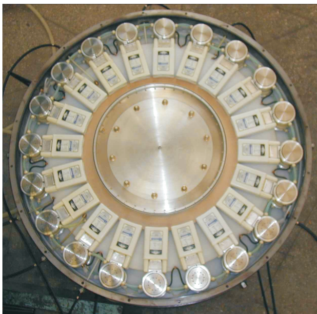
Fig. 9.10. Example of LTD module (0.45 MA, 100 ns) developed at High Current Electronics Institute, Tomsk, Russia [04Maz]. The module radius is about 1 m, and the module thickness is about 20 cm.
