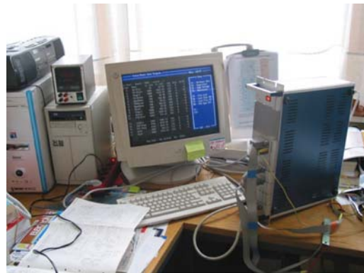
Fig. 23 & 24: In my lab: testing the automatic Test Box for the test of 3 \times 4160 cables for the ATLAS SCT detector.
