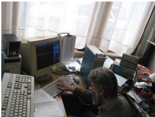
Fig. 23 & 24: In my lab: testing the automatic Test Box for the test of 3 \times 4160 cables for the ATLAS SCT detector.
