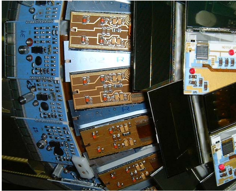
Fig. 17: The Very Forward Tracker silicon strip detectors (on the right) consisted of a total of 56 panes at each end. The panels were 5 \times 5 cm with a 5 \times 3 cm hybrid circuit supporting the readout chips (two 128 channel charge-sensitive amplifiers on each chip, with serial readout). Two such detectors were mouted back to back at 90^\circ so that the 256 active and 255 interpolation strips on each side formed a matrix. A high energy particle passing through (in \sim 5 ps) ionized the strips and after readout and computer analysis the trajectory could be reconstructed. The small red plastic balls were reference points for the LASER guided positioning and alignment of each detector (to < 20 \mu\text{m} ).
