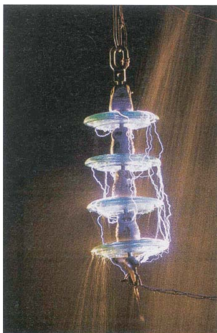
Fig. 9: Amazing what can be done by a single click of a humble 'mouse', isn't it? A four-element HV insulator gets a 270 kV surge, while under a heavy artificial shower. With a long photo exposure multiple breakdown partial discharge paths are revealed.
