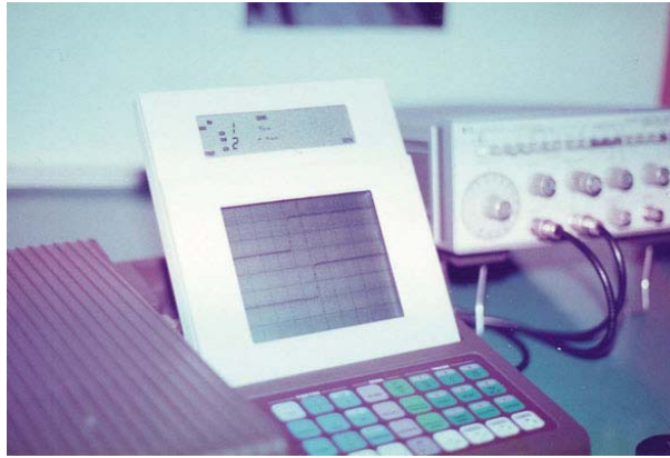
Fig. 2: Step response measurement and trigger delay in pre-trigger mode recording. In the background the HP-3312A function generator supplies the test signals. The input signal was fed either directly or through a 100:1 attenuator with a DC-GND-AC selector formed by 4 bi-stable relays driven directly from CMOS logic, to the Siliconix 2N5911 dual JFET source follower, followed in turn by two LF357 opamps (5 mV/div max. vertical sensitivity), driving the 1-2-5 attenuator sections, in addition to the offset and trigger-level controls using two AD7524 8-bit DACs. The ADC was a TRW TDC1001J 8-bit with successive approximation conversion, driven by a 20 MHz clock, sampling at 2 MHz in real time (and 10 MHz equivalent time in only 5 acquisition sequences, using a patented 5-step 200 ns ‘trigger shifting clock sync’ method of my own design, employing just 3 standard CMOS logic ICs). The time base could be set down to 50 s/div, allowing very slow events to be recorded.
