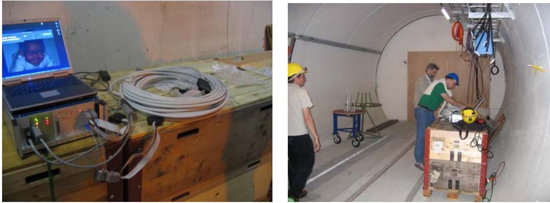
Fig. 25 & 26: Testing the first bunch of cables in the tunnel behind the ATLAS cavern. The cable (four power lines, four sense lines, two HV lines, six control lines, and a shield) is tested for connectivity identification, insulation ( 20\text{ M}\Omega ), line resistance (to 5\text{ m}\Omega resolution), and for HV leakage (to 1\text{ nA} at 500\text{ V} ). My colleague Gregor Kramberger wrote the PC software (and his 18 months old daughter Živa supervises the test operations from the laptop screen).
