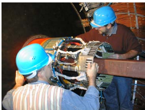
Fig. 15 & 16: The Vertex detector. The silicon pixel detector forms a barrel, whilst the Very Forward Tracker is on both ends.
