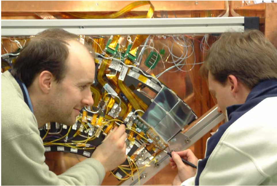
Fig. 22: Part of the ATLAS SCT (Silicon Tracker) on the test bench. The detector modules have 6 readout chips, each of 128 channels. The power and control signals are supplied by thin Al on Kapton tapes (up to 4.5 m long), designed at IJS and produced by Elgoline, a Slovenian PCB production company (aluminum is used because it is not activated by radiation, unlike Cu). The readout is performed through optical links (the thin yellow cables).
