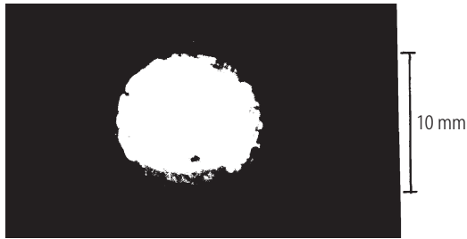
Fig. 8.1.8. Photograph of the beam profile of a Nd:YAG rod laser ( \lambda = 1.064 \mu\text{m} ) with a stable resonator in multimode operation (maximum of 2p + l + 1 is about 60) [97Hod].
