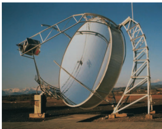
Fig. 4.1.38. Dish Stirling built by Schlaich, Bergermann and Partner (SBP). The collector is built as a stretched membrane coated with thin glass mirrors. The sunlight powers a Stirling engine (source: SBP).
