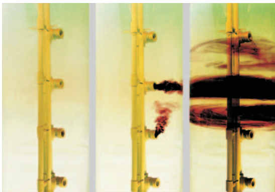
Fig. 4.3.6. Dyed water entering a stratified tank (storage: Solvis Energiesysteme GmbH, Braunschweig).
